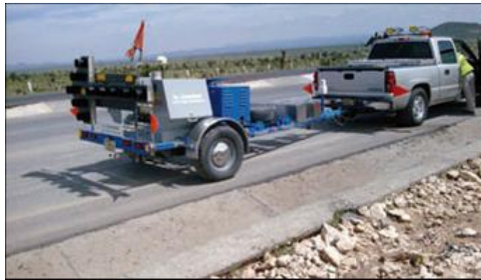
Figure 4 - Pavement deflections being measured with HWD equipment in a toll-free federal road (Osio, 2010).
