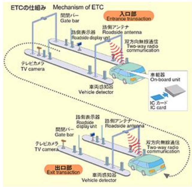
Figure 4.1.9 - ETC mechanism
