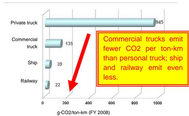
Figure 4.5.2 - CO<sub>2</sub> emissions per cargo volume by transport mode
