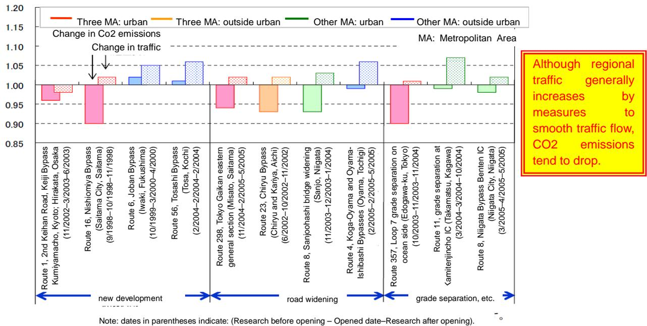
Figure 4.1.5 - Changes in CO<sub>2</sub> emissions due to bypass construction, lane widening, and intersection grade separation
