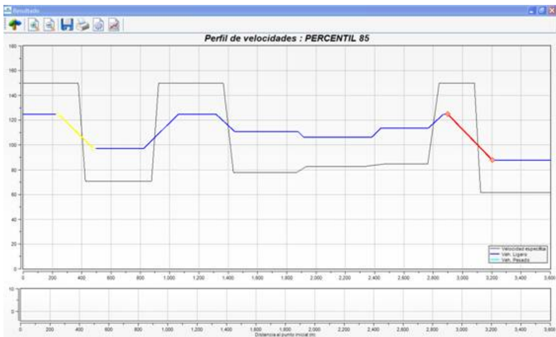
Figure 7 Graph of results of the analysis programme of the consistency of the road
