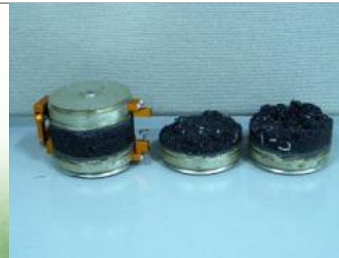
Prepared Sample (above) and Sample After Test (below)
