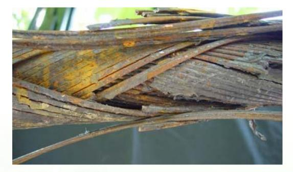
A severly damaged strand under clip n°8 after removal
