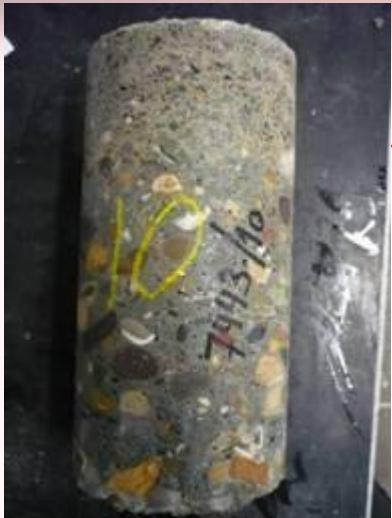
double layered concrete with recycled concrete aggregates in base layer and photocatalytic concrete in top layer on industrial zone “Den Hoek” in Wijnegem
