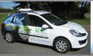
Calibration: MRT (vehicle Ifsttar: VERT) Cinematic bi-frequency GPS\_& inertia station, accuracy: a few cm
