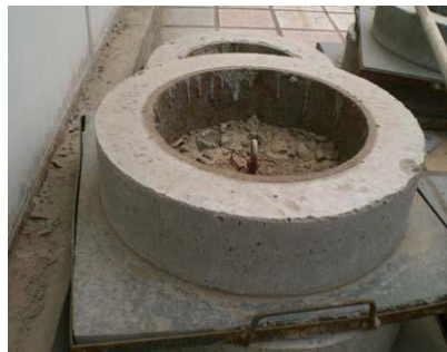
Figure 3-Schematic of Ring Set Up for Concrete crack test
