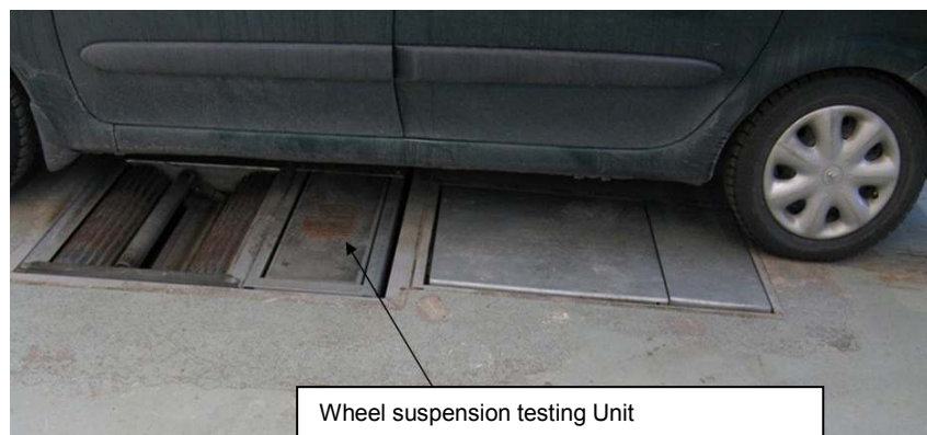
Figure 4. Equipment with vibration plates was used to study the effect of tyre pressure.
