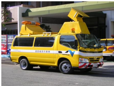
Figure 2 - HDV-Equipped Inspection Vehicle Figure 3 - Mechanism of Image Processing
