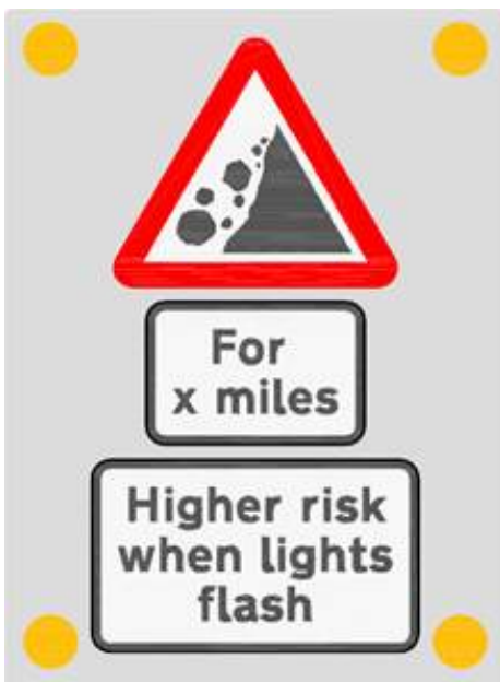
Figure 6 – Landslide wig-wag sign.
