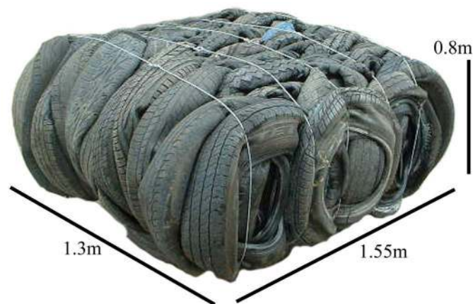
Figure 1 – A typical tyre bale with dimensions.
