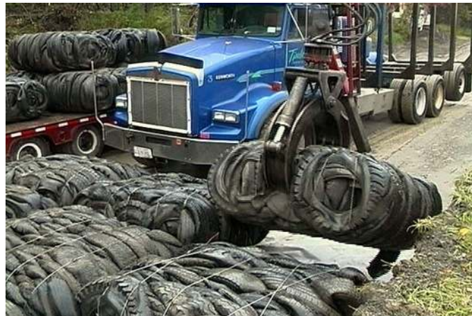
Figure 6 – Use of a 'loggers'-clam' to handle tyre bales. (Photograph courtesy of Ken Smith, Chautauqua County Department of Public Facilities, New York State).
