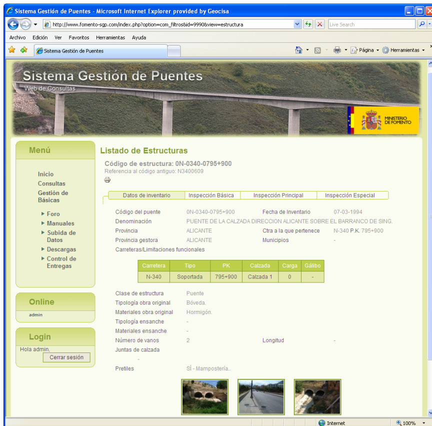
Figure 6 – Query web page. Display of inventory data of a bridge.
