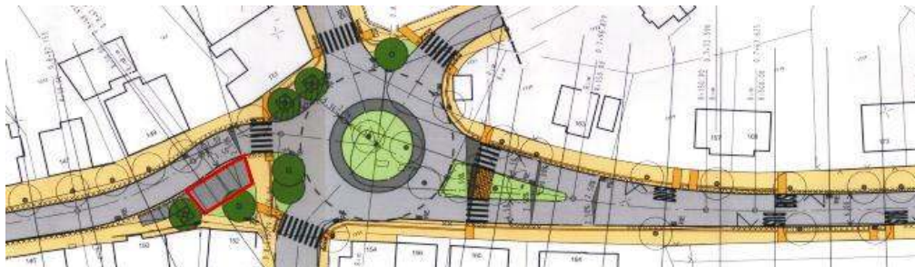
Figure 3: Sight obstructions at pedestrian crossings caused by parking vehicles
