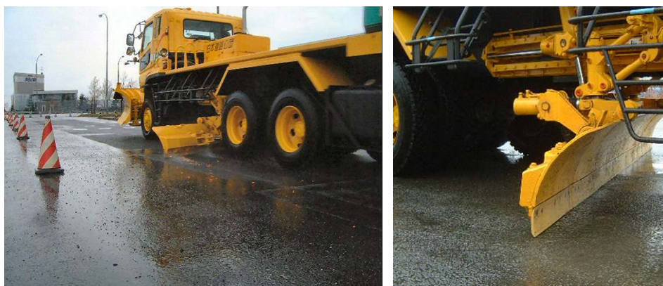
Photo 5 - Steel ploughing abrasion test
