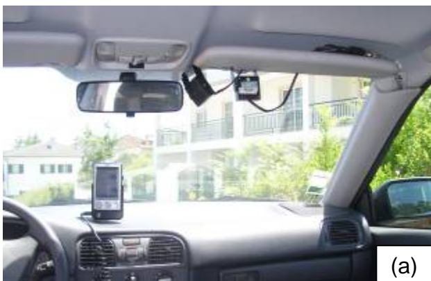
Figure 7 – Lateral and front view cameras (a); rear view camera (b)
