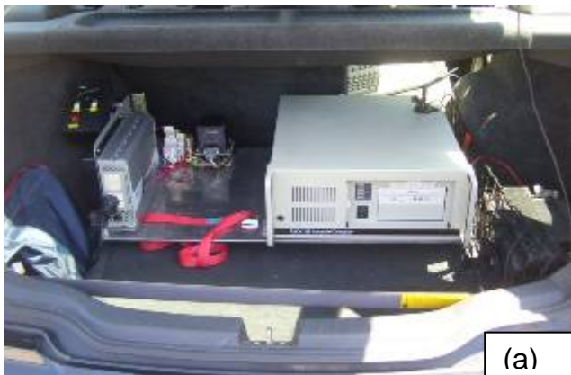
Figure 6 – Computer and support systems in the vehicle trunk (a); interface (b)
