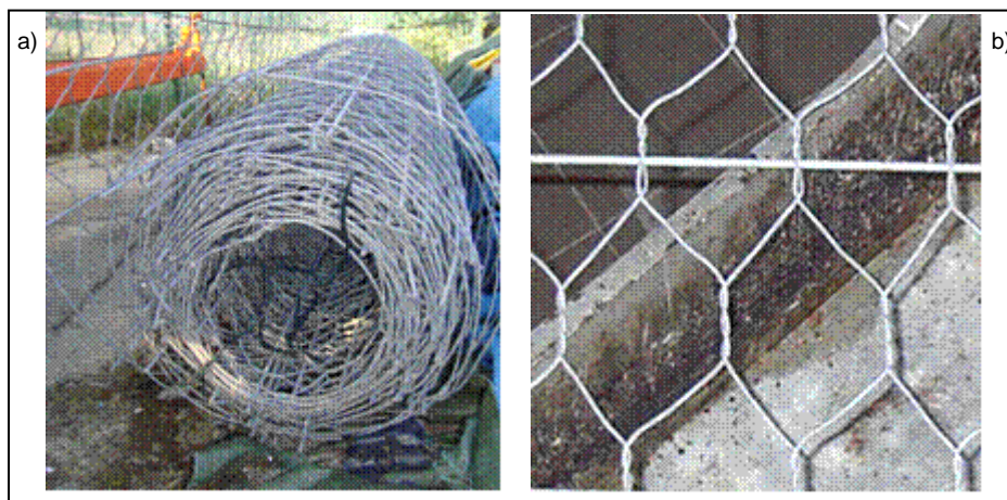
Figure 4 - Steel net reinforcing system (a) and a detail of the double twisted grid (b)
