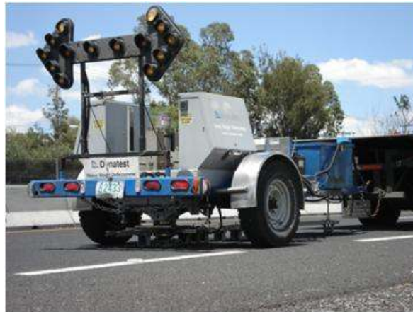
Figure 2 - Deflection measurements using a falling weight deflectometer in the federal network.
