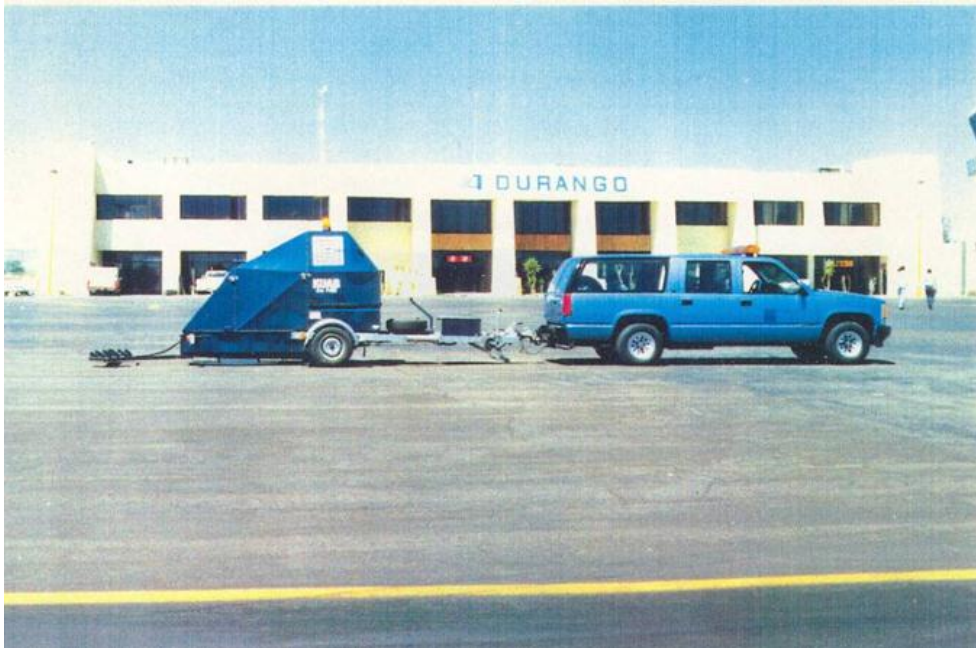
Figure 5 - Deflection measurements with FWD in Durango Airport. "Inverted section" pavement
