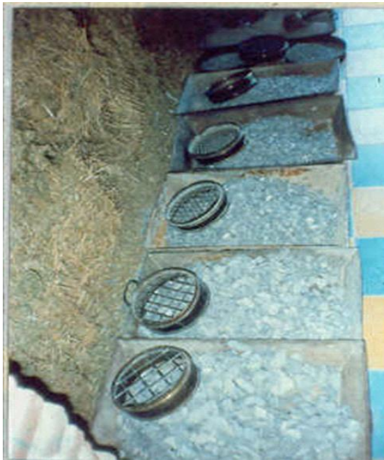
Figure 6 - Solids elements of CCR in sub-base course. Guadalajara-Colima highway. Portland cement content: 10%; water/cement. ratio: 0.37 \pm 0.03 ; elastic modulus: 7000 MPa. Crushed basaltic gravel
