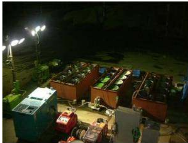
Photo 4 - Thermostat and measuring tanks for epoxy resin
