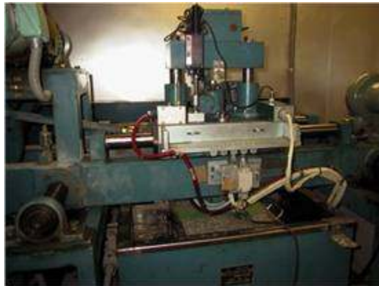
Photo 1 - Wheel tracking test
