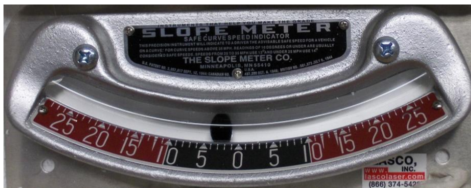
Figure 3 - Safe Curve Speed Indicator
