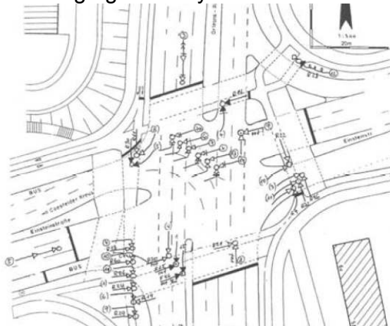
Figure 6 - avoidable safety deficits caused by missing safety measures for participants turning left at traffic signals [7]
