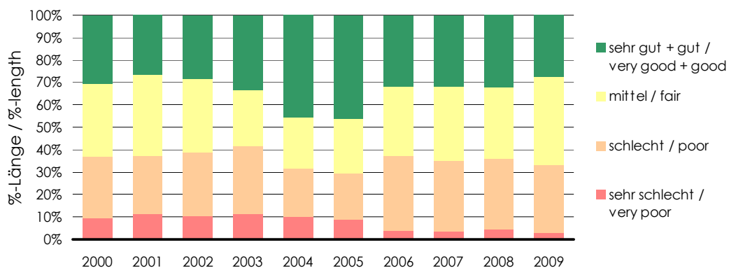
Figure 6: Condition distribution total condition index pavement [2]
