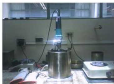
Asphalt disperser La Salle University Laboratory
