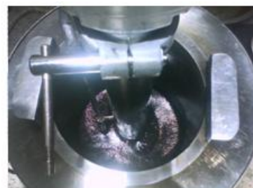
Asphalt disperser La Salle University Laboratory
