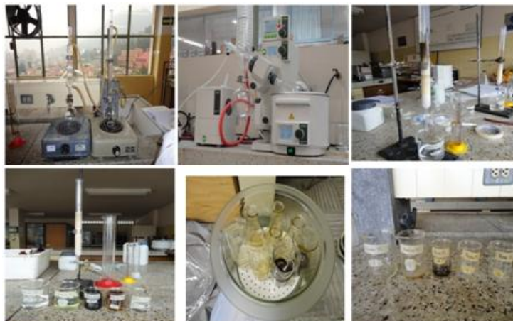
Figure 3 Separation of the asphalt into its four SARA (Saturates, Aromatics, Resins, Asphaltenes) fractions.
