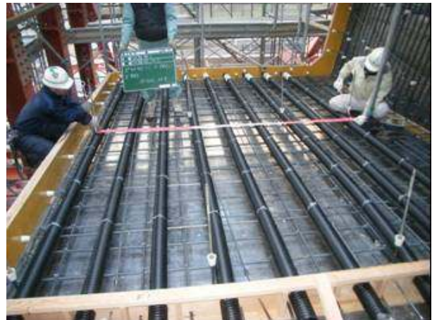
Photo 3 - Full-scale specimen (slab)
