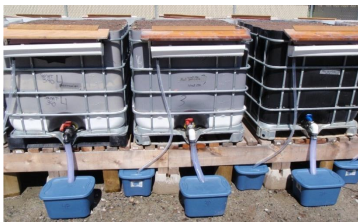
Figure 3 – Runoff and percolation water reclamation systems at Laval University
