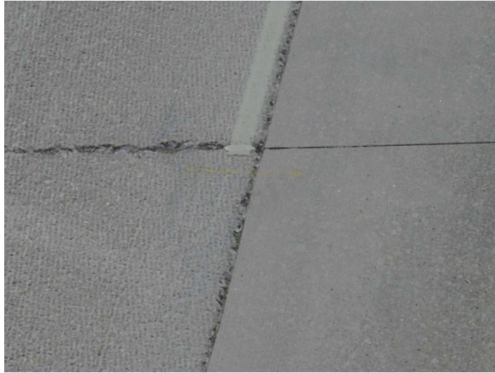
FIGURE 9. Difference between micro-milling (left) and diamond grinding (right).
