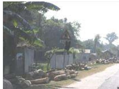
Fig.9: Loading of vehicles, piled logs on the roadway shoulder creating serious hazards & visibility obstructions-informative sign ('school ahead') is hardly visible due to adjacent land developments
