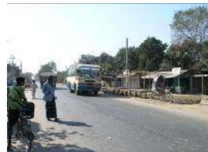
Fig.10: Unloading of passengers on the through lane of the high speed road and temporary shops fronting the main road create severe road safety
