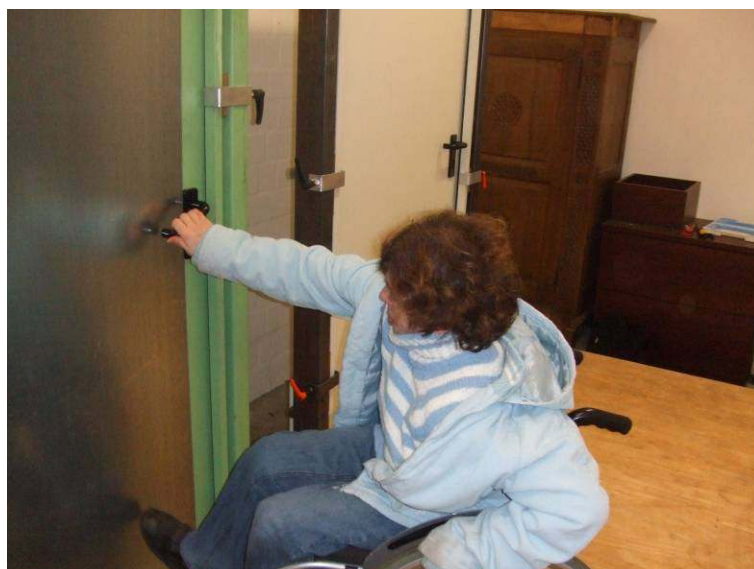
Figure 6 – Handicapped person on test circuit to scale the power one could effort to open fire protection doors in road tunnels [5]
