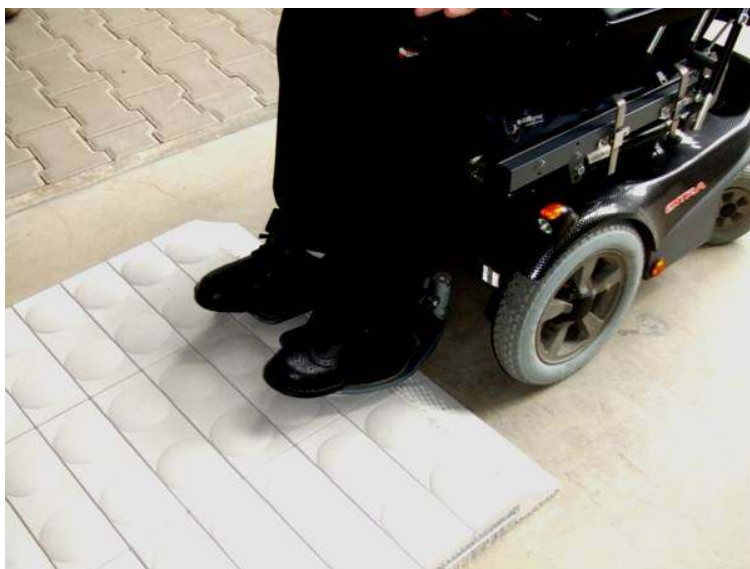
Figure 4 – Example for tactile elements to be used in front of exit doors (test area during the research) – accessibility by wheel chairs is a must
