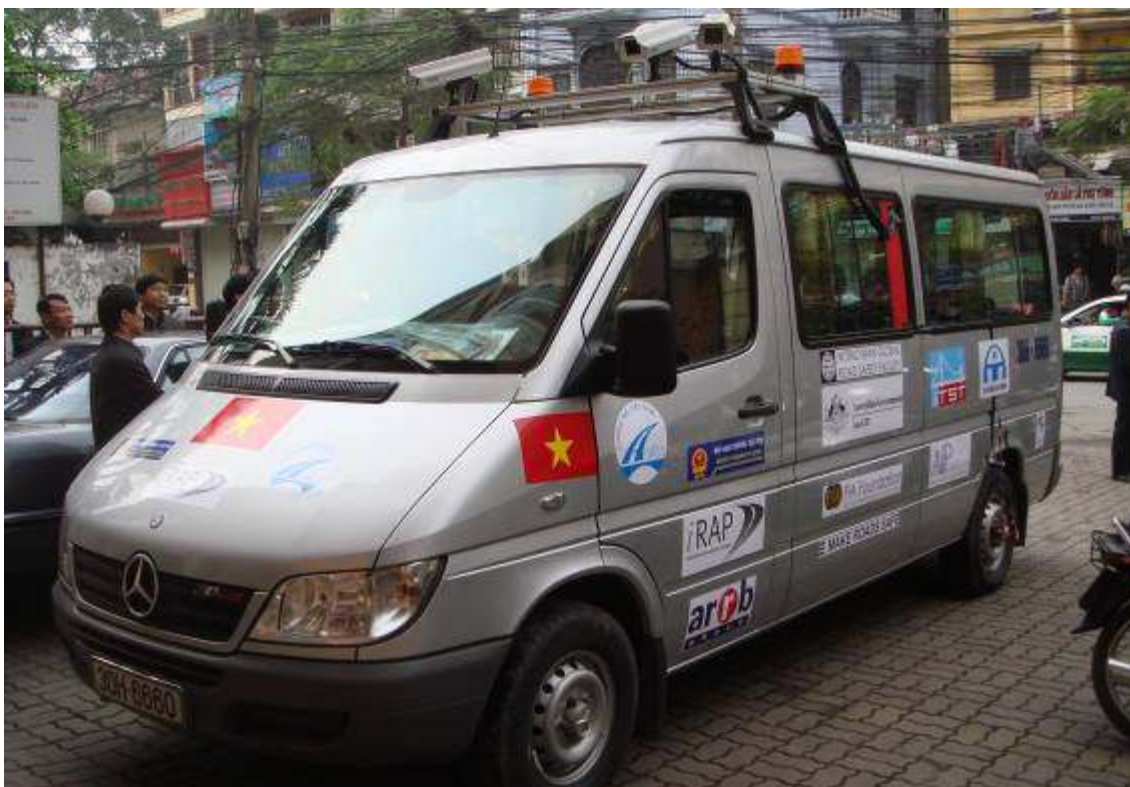
Figure 1 - The iRAP Vietnam inspection vehicle
