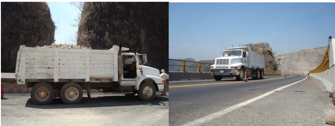
Figure 8 – Lorry before and during the load test
