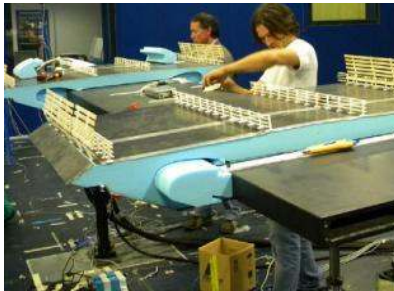
Figure 23 - Wind Tunnel Testing : deck section and balanced cantilever from central tower
