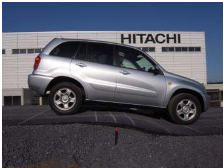
Photographs 15 - Trafficability test on asphalt pavement on CRE after 300mm forced settlement
