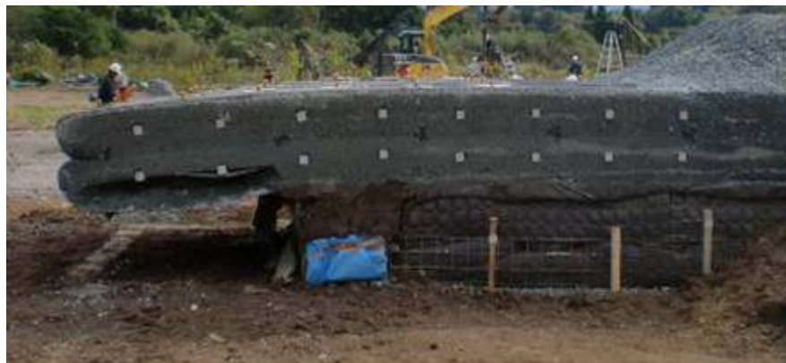
Photograph 11 - Cantilever model test (0.5m thickness, 1.5m span)
