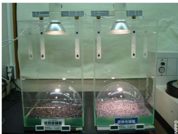
Figure 20 – Laboratory tests on atmospheric temperatures(left: conventional, right:S.H.P.)
