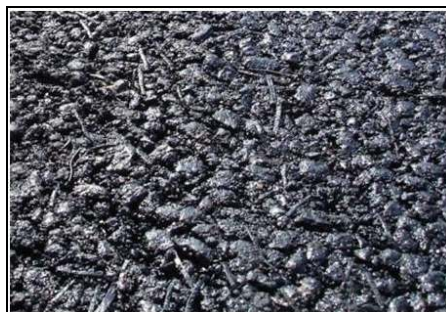
Figure 5 - Close-up surface of mono-strand fiber-reinforced HMA
