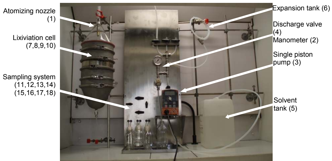
Figure 2 - Picture showing the experimental extraction system by lixiviation
