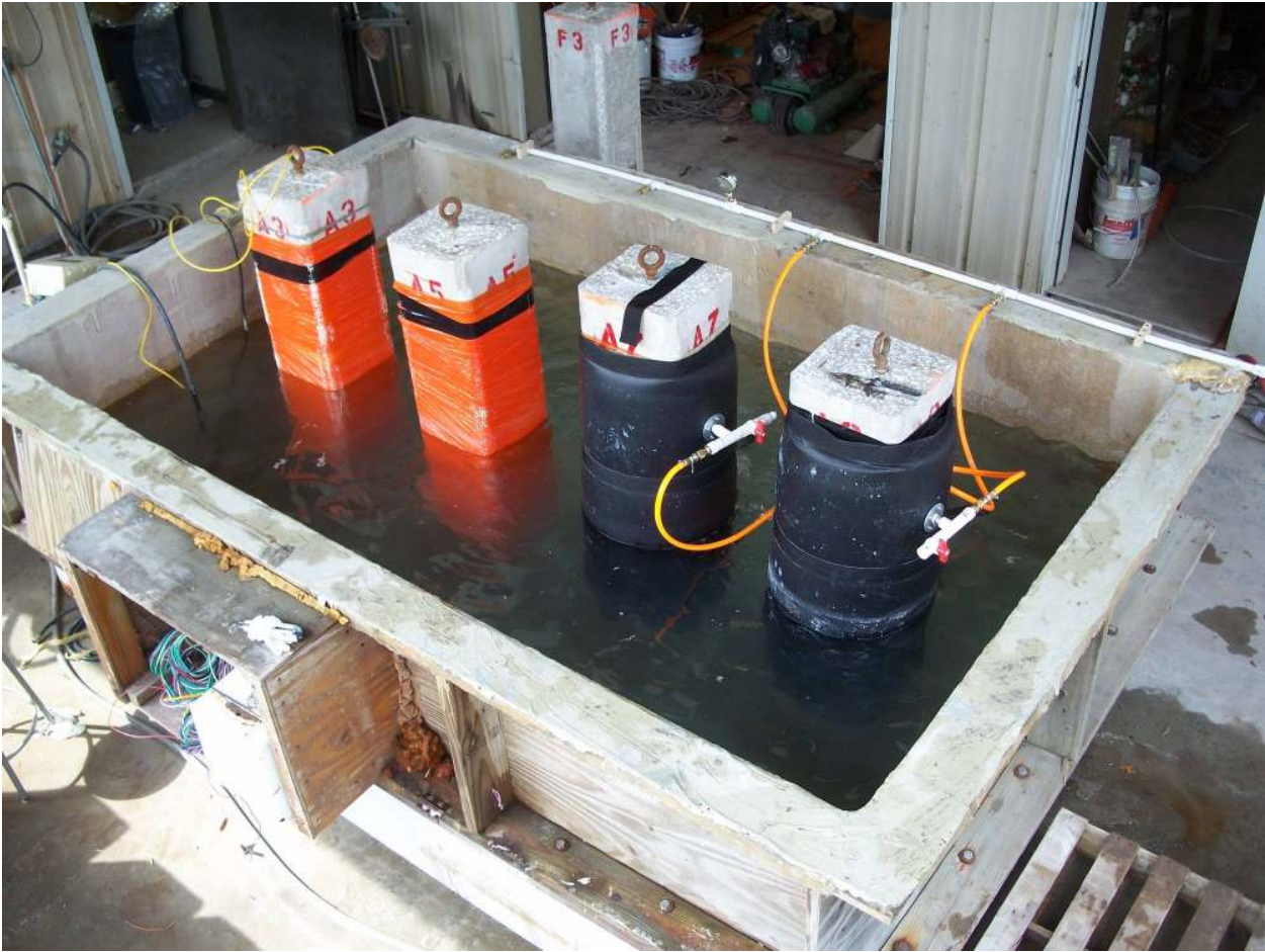
Fig. 4 Current practice vs pressure bagging
