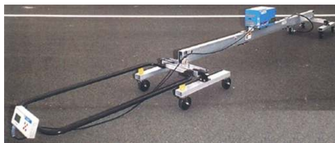
Figure 3-17 Road Surface Profile Measure
