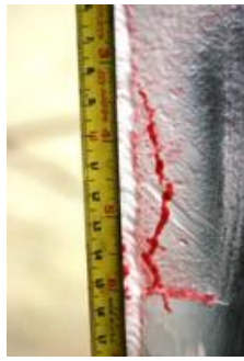
(b) Element Id. No. 7 Large grain size
