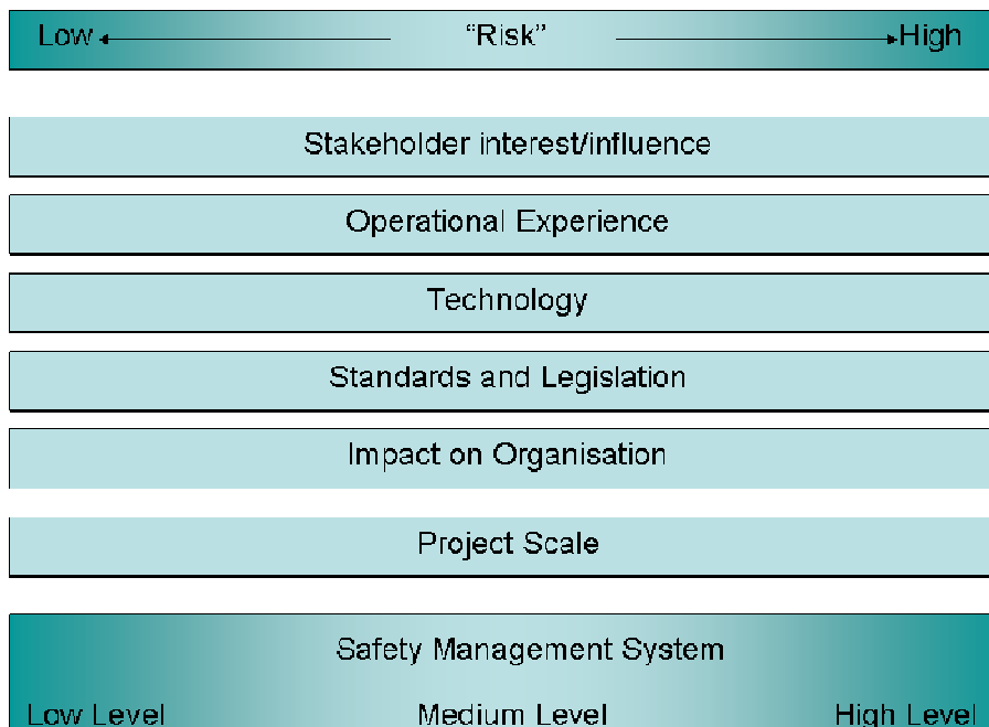
Figure 2: Typical features used to categorise a project’s SMS requirements
