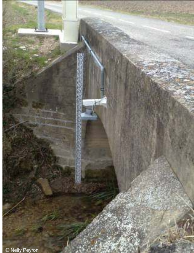
Figure 12 – Automatic gauging station with telemetry system incorporated, installed within the TRACE project.
