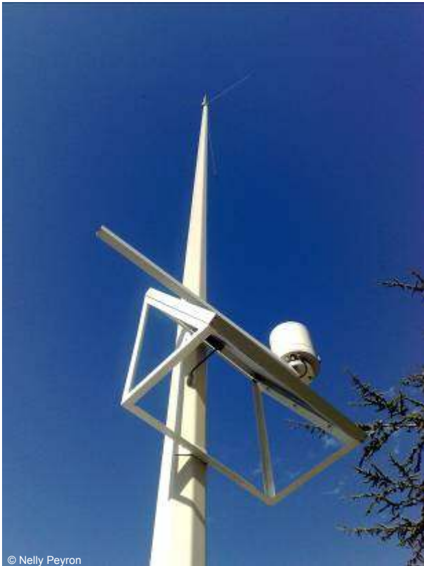
Figure 12 – Automatic gauging station with telemetry system incorporated, installed within the TRACE project.
