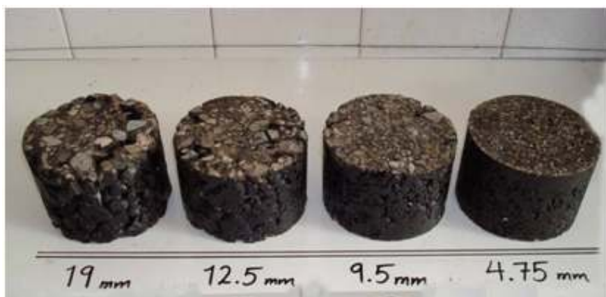
Figure 2- View of different laboratory prepared specimens (SMA & HMA).
