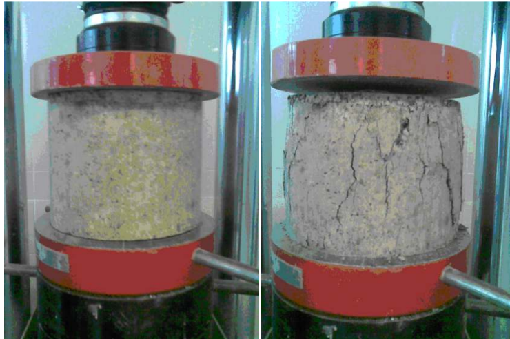
Figure 6 – Sample before (left) and after (right) compressive strength tests according to standard HRN EN 13286-41
