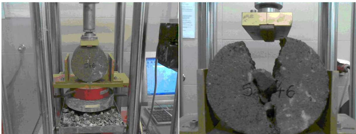
Figure 7- Sample before (left) and after (right) tensile strength tests according to standard HRN EN 13286-42
