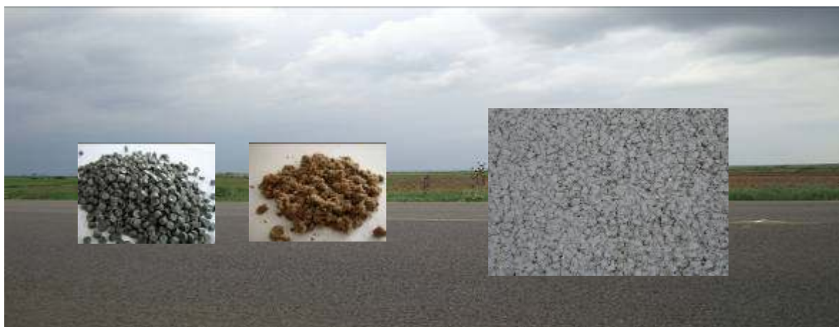
Figure 10 - Modified asphalt mixture MM with granulated polymers and fibres
