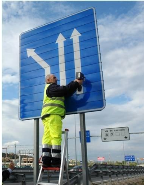
Figure 1 - Measuring with a hand-held retroreflectometer
