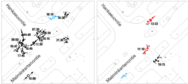
Figure 4 - Accidents before installation of signalization to the left and accidents after installation of signalization to the right.
