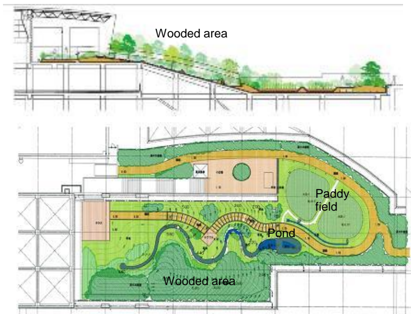
Figure 15 – Roof Garden on the Ventilating Station
