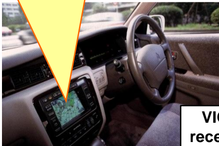
Traffic congestion guidance using VICS (Vehicle Information and Communication System)
