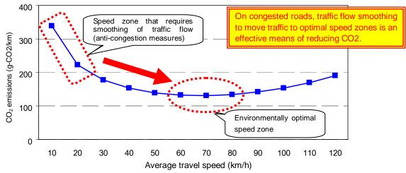
Figure 4.1.1 - The relationship between travel speed and CO<sub>2</sub> emissions
