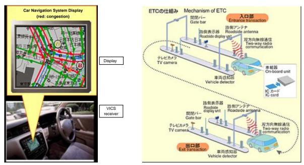
Figure 4.1.8 - Traffic congestion guidance using VICS
