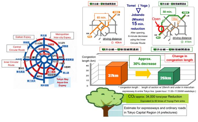
Figure 4.1.6 - Status of construction of the three ring roads in Tokyo metropolitan area (Blue: as of April 2010; Red: not yet completed)
